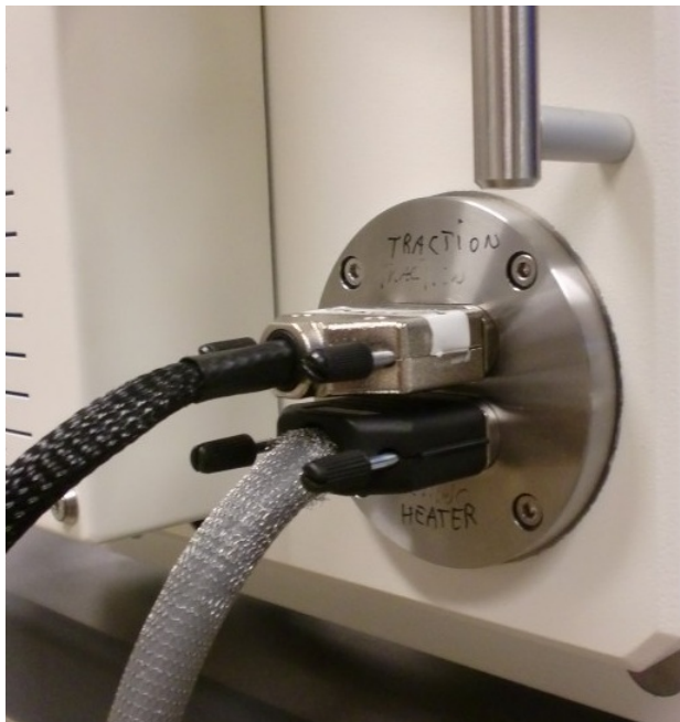
Figure 14: Connect the cables from the movable computer. Traction in the upper contact and heating in the lower contact.
