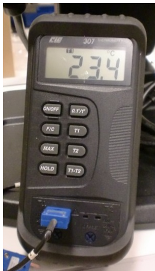
Figure 15: Test the thermocouple and make sure it responds by squeezing it with your fingertips.
