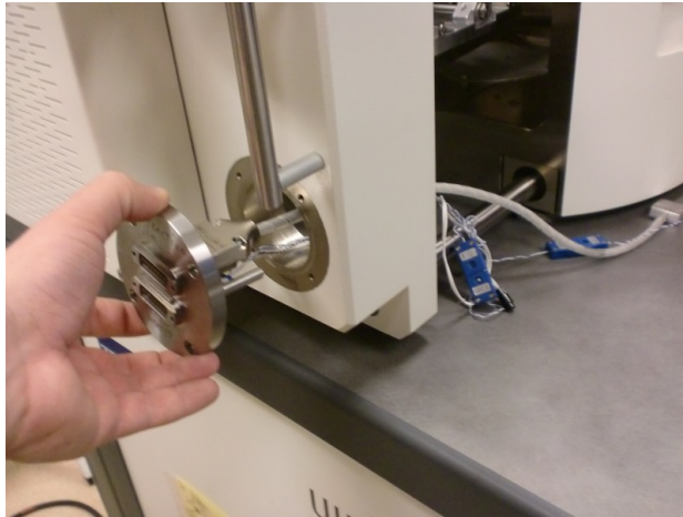
Figure 13: Mount the tesile stage cable and thermocouple to the door contact, lead the cables through the door and screw the contact to the door.
