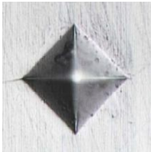
Figure 4.1: Resulting indentation from a Vickers hardness test [9]
