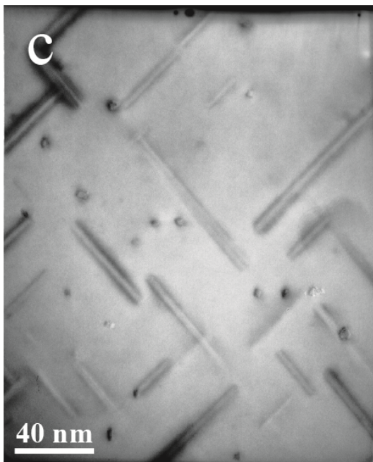
Figures C.16 (a)-(d): Examples of TEM images taken with Philips CM30 at local max at overaged conditions after artificial ageing at 200 °C for KK6 at 420k magnification
