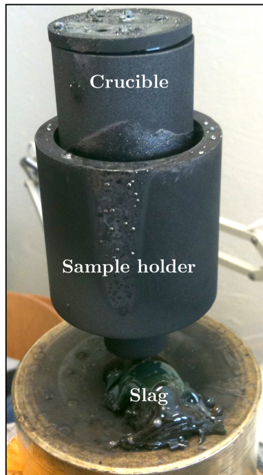
Figure 4.9: The sample holder with crucible after the Slag 1, 1650 °C experiment. The sample holder is in the lowered position.
