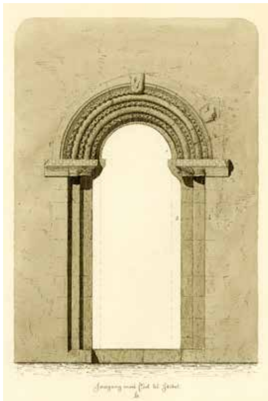
Figure 2. The old west portal in the nave of Dønnes church as it was drawn in 1860 by C. Christie before the church was rebuilt in 1866. The frame of the portal with its ornamentation is made of soapstone. (©The Directorate for Cultural Heritage, The Archive).
