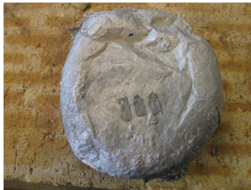
Figure 4.8 The oxide skin left in crucible after melting
