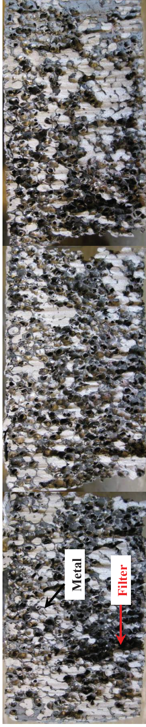
Figure 4.39 Cross sectional view of the spent filter in Exp.4 - SiC industrial filter Black parts are filter materials.
