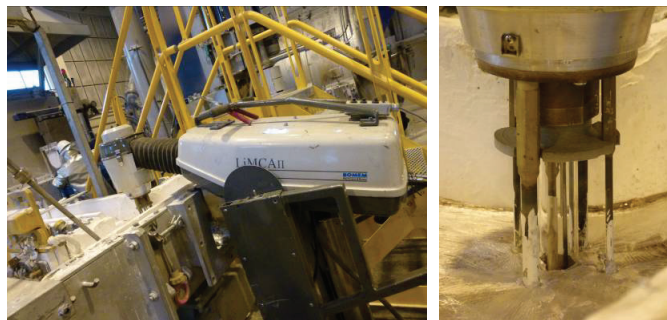
Figure 4.4 LiMCA II in operation, positioned after the filter
