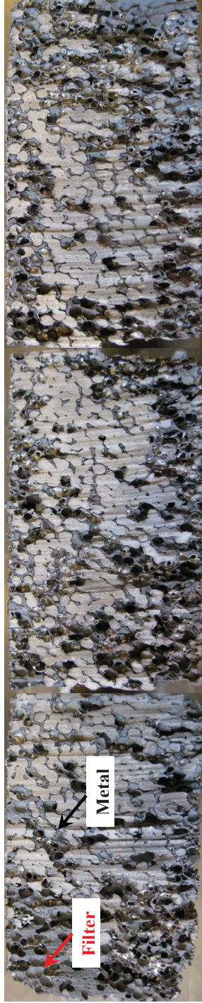
Figure 4.37 Cross sectional view of the spent filter in Exp.2 - SiC industrial filter Black parts are filter materials.
