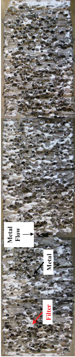
Figure 4.36 Cross sectional view of the spent filter in Exp.1 - Al 2 O 3 industrial filter White parts are filter material.
