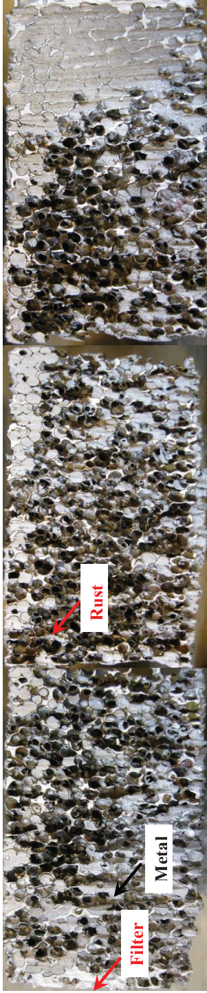
Figure 4.38 Cross sectional view of the spent filter in Exp.3 - \text{Al}_2\text{O}_3 industrial filter White parts are filter material, red is rust from saw.
