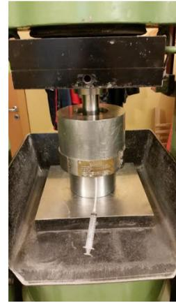
(b) Setup for pore solution extraction.
