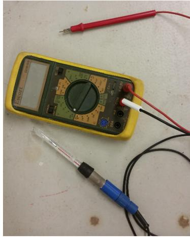
Figure 19: Setup of corrosion potential measurement.
