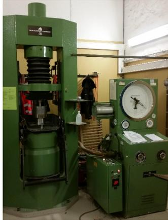
(a) The machine used for pore solution extraction.
