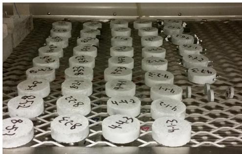
Figure 14: Bottles sawn into discs, placed in carbonation cabinet.
