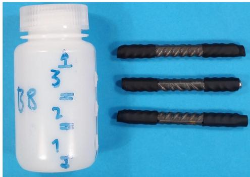
Figure 18: Reinforcement bars and bottle before mounting
