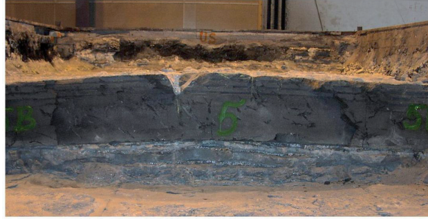
Figure 3.19: Photographs of the cathode heave of a 585 days old pot [3].
