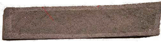
Figure 4.2: The cross section of virgin Block A. The area closed to the block surface has lighter color than the center area.
