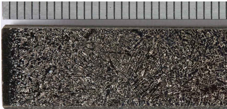
Figure 4.13. Macrostructure of casting 5. (Scale bar unit 1mm.)
