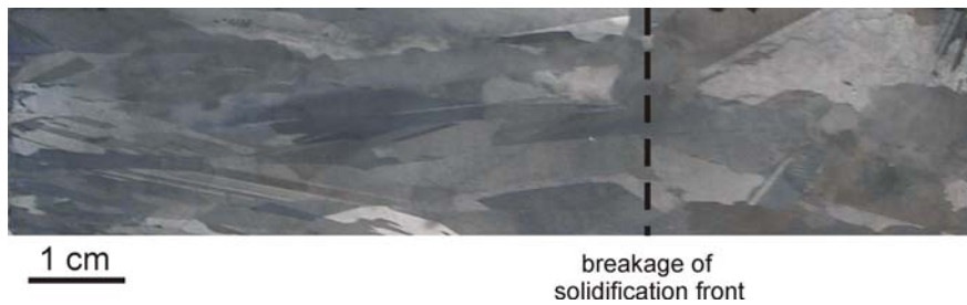
Figure 5.3: Breakage of the planar solidification front to cellular front in the upper 2 centimeters of the ingot FS-4B.
