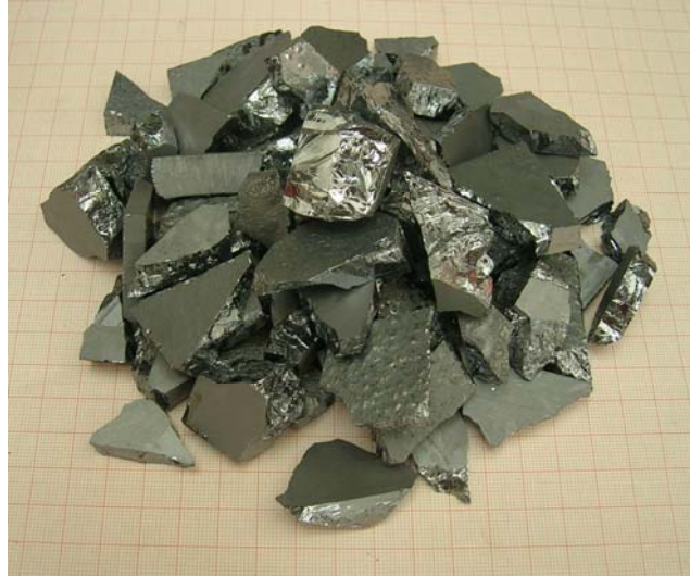
Figure 3.18: Top cut silicon scrap as used in filtration experiments. The square piece of silicon scrap was broken into smaller pieces before it was filtered.
