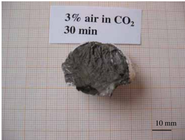
Figure 2.25 Sample exposed to 3% air in CO 2 , series 3. See Table 2.3 and 2.11, 30 minutes.
