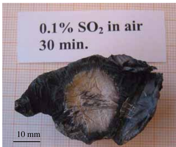
Figure 2.15 Sample exposed to 0.1% SO 2 in air for 30 minutes. See Table 2.2 and 2.8.
