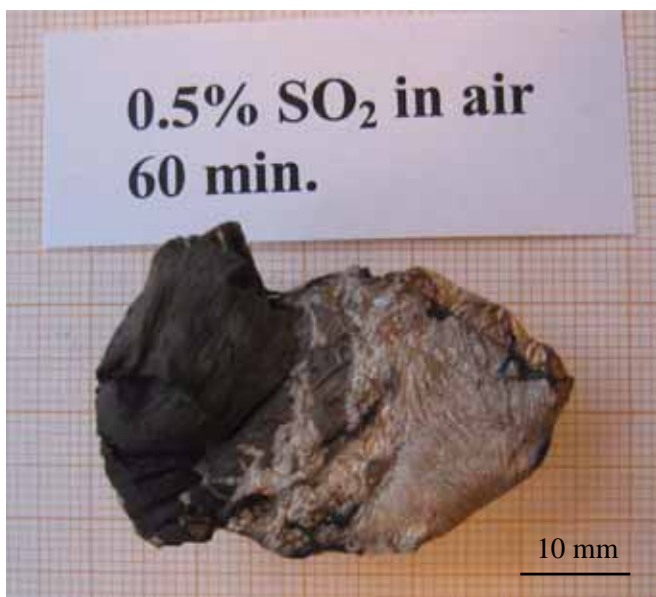
Figure 2.13 Sample exposed to 0.5% SO 2 in air for 60 minutes. See Table 2.2 and 2.8.
