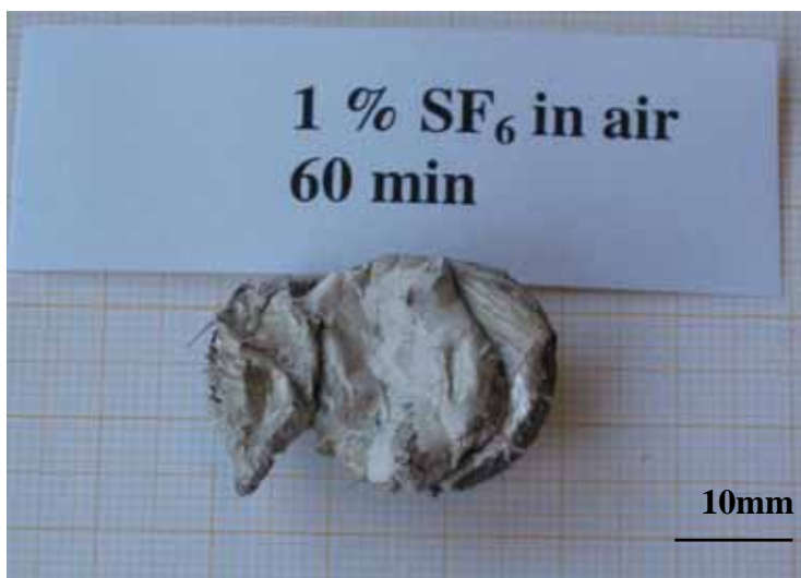
Figure 2.3 Sample exposed to 1% SF 6 in air, series 2. (See Table 2.1 and 2.4, 60 minutes.)
