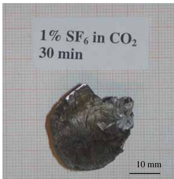
Figure 2.9 Sample exposed to 1% SF 6 in CO 2 . See Table 2.1 and 2.7, 30 minutes.
