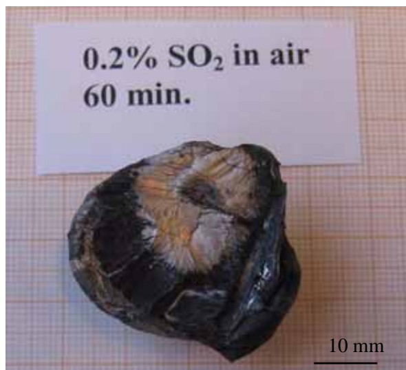
Figure 2.14 Sample held in 0.2% SO 2 in air for 60 minutes. See Table 2.2 and 2.8.
