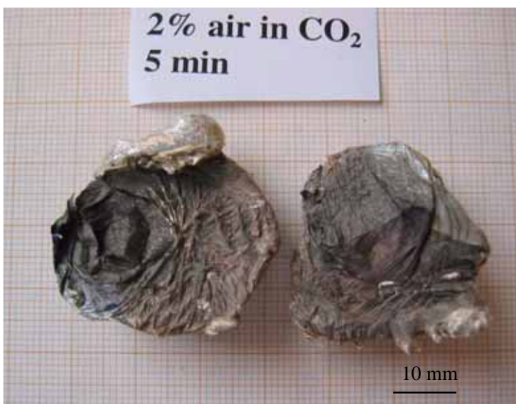
Figure 2.24 Two samples exposed to 2% air in CO 2 , series 3. See Table 2.3 and 2.11, 5 minutes.
