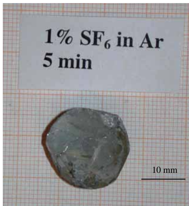
Figure 2.7 Sample exposed to 1% SF 6 in Ar. No protective film is formed. See Table 2.1 and 2.6, 5 minutes.
