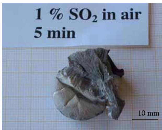
Figure 2.11 Sample exposed to 1% SO 2 in air, series 2. See Table 2.2 and 2.8, 5 minutes.
