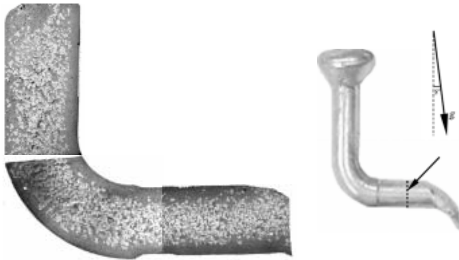
a) Figure 6: a) Macrographs of a longitudinal section of an A356 casting produced with T_{die}=270^{\circ}\text{C} and f_s\sim 0.16 . The ESCs appear as large primary dendrites (white). The fine grains and the Al-Si eutectic comprising the matrix appears as dark grey; b) A photograph of the casting. Microstructural samples were taken from the plane marked with an arrow.
