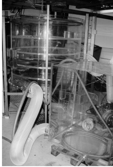
Figure 1.11: Photograph of the water model of the vortex chamber. The cubic container in the front is the reservoir while the vortex chamber is in the background. The flowmeter was not installed when the picture was taken.
