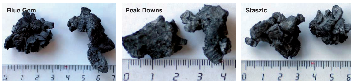
Figure 5.38: Best suited particles for TG experiments.
