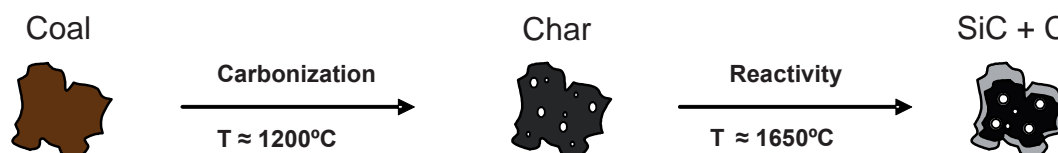
Figure 5.1: Progress of this work can be divided into three distinct parts: 1) Evaluating material properties of the selected coals. 2) Carbonizing coals and determining material properties of the carbonized material. 3) Testing the carbonized materials in the SINTEF \text{SiO} reactivity apparatus and evaluating the results.
