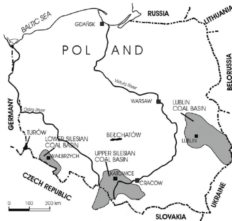
Figure 4.18: A map showing the coal deposits in Poland. The shaded areas indicate the resources of high rank coals. Lignite deposits located in Bełchatów and Turów are marked in black. Figure modified after Kotarba and Lewan (2004).
