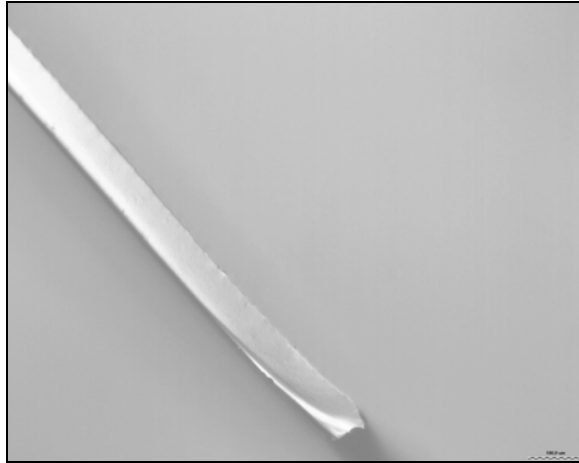
Figure 7-2 Magnified image of the cross section of a carbon flat sheet membrane (cellulose with 4 wt% copper (II) nitrate, carbonized at 650°C under vacuum)
