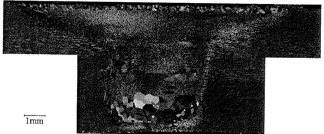
Figure 11 Microstructure of post weld annealed AA7108.50-T79, 30 min at 475°C.
