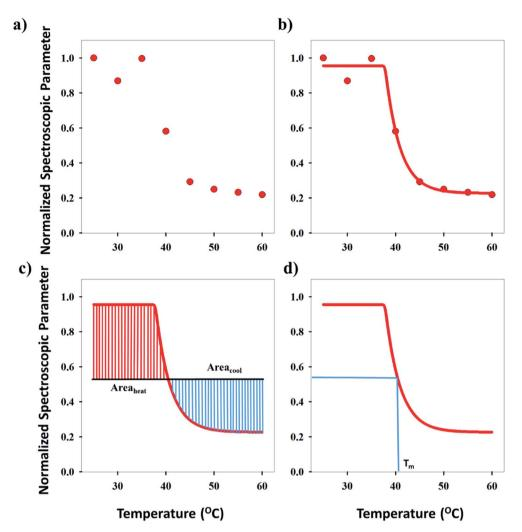
Fig. 1 Schematic showing calculation of VPTT. (a) Normalized spectroscopic parameter as a function of independent variable (temperature, °C). (b) Fitting of Sigmoid, 5 parameter curve to the experimental dataset. (c) Area equalization algorithm. (d) Determination of VPTT using MATLAB® code.
