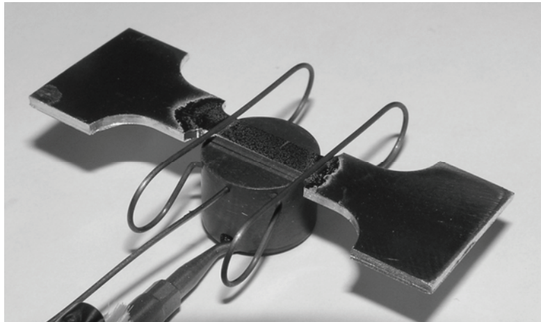
Figure A.1 – Small furnace clamped to the specimen. The specimen can easily be mounted in the deformation stage.
