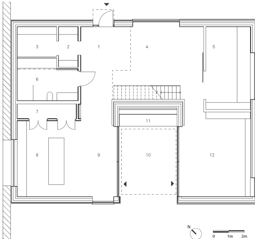
Figure 2.3 Ground floor plan, with entrance (nr. 1), wardrobe (nr. 2), store (nr. 3), multi-media room (nr. 4), office (nr. 5), bathroom (nr. 6), technical room (nr. 7), kitchen (nr. 8), dining room (nr. 9), atrium (nr. 10), fire shelf (nr. 11), lounge (nr. 12). Source: Snøhetta.
