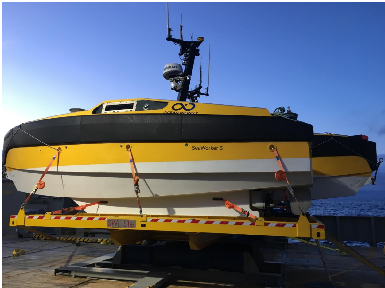
Fig. 7. C-Worker 7 Ocean Surveying ASV. Photo: Anna Lim.
