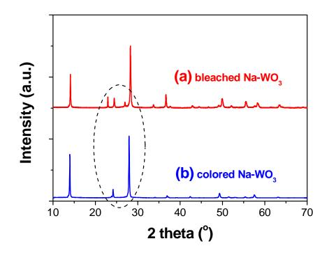
Figure 8. (color online). XRD patterns of the as-prepared Na-WO<sub>3</sub> nanorods at (a) bleached and (b) colored state. The XRD patterns are shifted vertically for clarity. Dashed circle highlights the differences between the two patterns.
