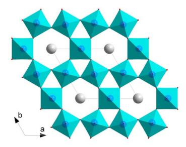
Figure 1. (color online). Polyhedral representation of hexagonal sodium tungsten bronzes Na-WO<sub>3</sub>. The structure is viewed down the c axis of a hexagonal unit cell. Tunnel species (Na<sup>+</sup> ions and water molecules) are represented by grey spheres.
