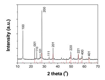
Figure 2. (color online). XRD pattern of the as-synthesized materials. The bars at the bottom represent the calculated diffraction pattern of hexagonal Na-WO<sub>3</sub> (JCPDS 81-0577). Miller indices are given to the main reflections.
