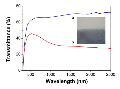
Figure 7. (color online). Transmittance spectra of the as-prepared Na-WO<sub>3</sub> nanorod electrode at (a) bleached and (b) colored state. Inset shows an optical photograph of the corresponding sample.
