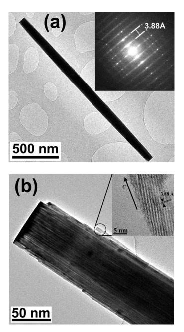
Figure 4. TEM images of the as-prepared Na-WO<sub>3</sub> nanorods. Inset of panel a shows the corresponding ED pattern. Inset of panel b shows a high-resolution lattice image of a Na-WO<sub>3</sub> nanorod.
