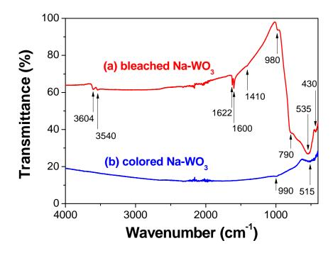
Figure 9. (color online). FTIR spectra of Na-WO<sub>3</sub> nanorods at (a) bleached and (b) colored state. The noise around 2000 cm<sup>-1</sup> is due to the ATR diamond crystal.
