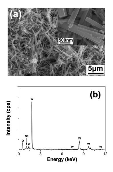
Figure 3. (a) SEM images and (b) EDS spectrum of the as-prepared Na-WO<sub>3</sub> nanorods.
