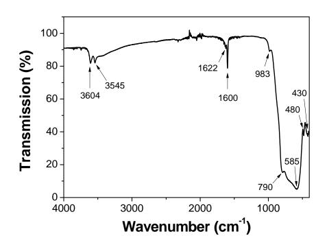
Figure 5. FTIR spectrum of the as-prepared Na-WO<sub>3</sub> nanorods. The noise around 2000 cm<sup>-1</sup> is due to the ATR diamond crystal.
