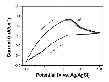
Figure 6. Cyclic voltammetry (CV) curve of the as-prepared Na-WO<sub>3</sub> nanorods in 1 M H<sub>2</sub>SO<sub>4</sub> aqueous solution. Arrows show the scan direction. Scan rate: 50 mV/s.
