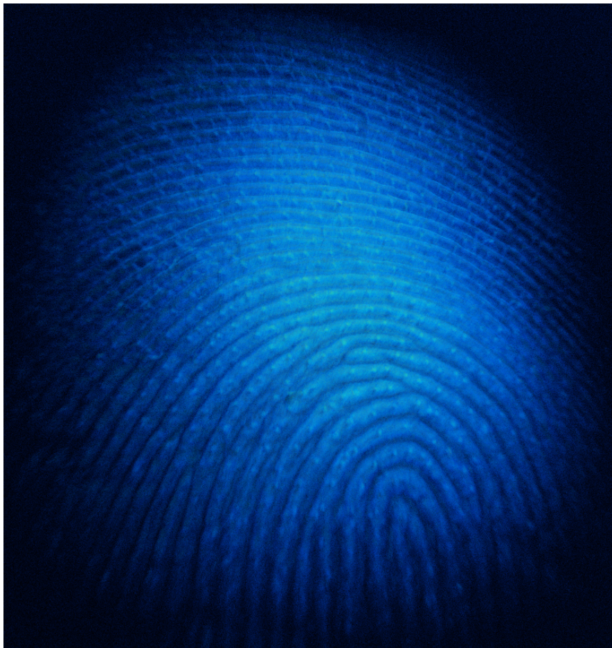
Figure 4.7: OCT scanner 2.0; thumb scan: 2x2cm area, 1408x1408x1024, 14.2 \mu m - sweat glands overview - transparent 3D visualization
