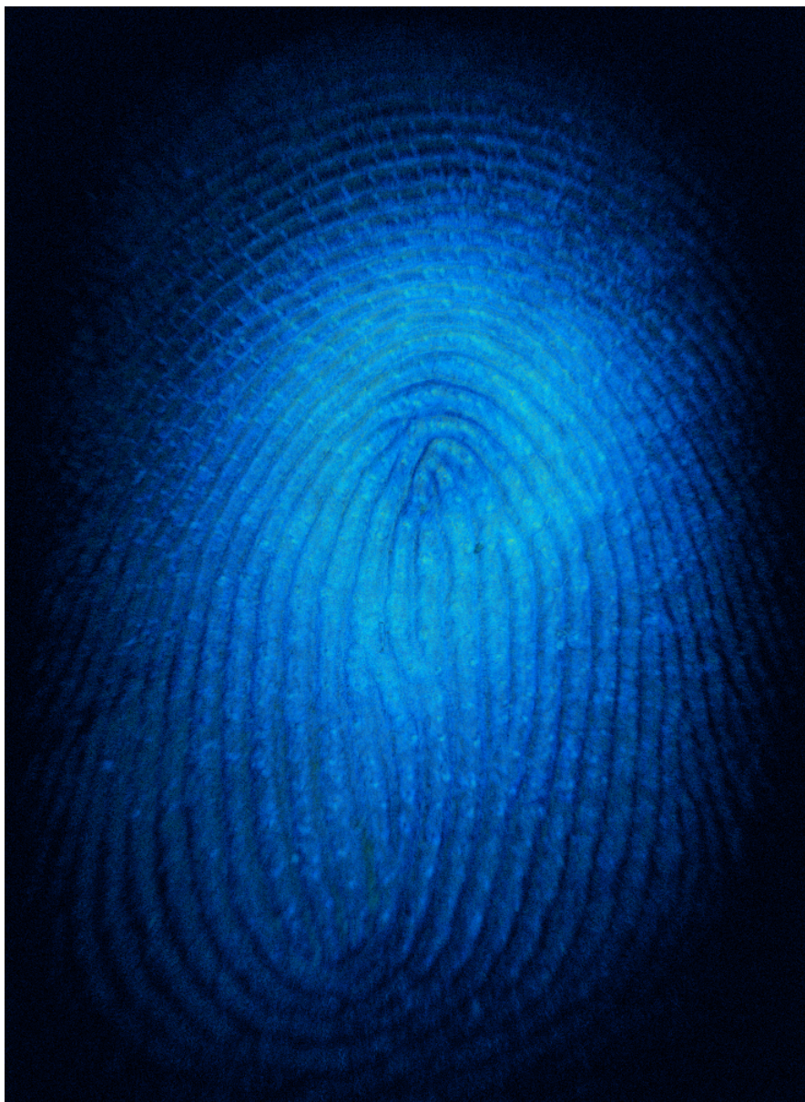
Figure 4.5: OCT scanner 2.0; index finger scan: 2x2cm area, 1408x1408x1024, 14.2 \mu m - sweat glands overview - transparent 3D visualization
