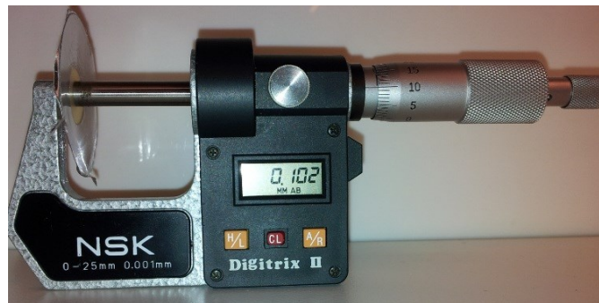
Figure 6.9 Digitrix II Disc Micrometer used to measure the membrane thickness
