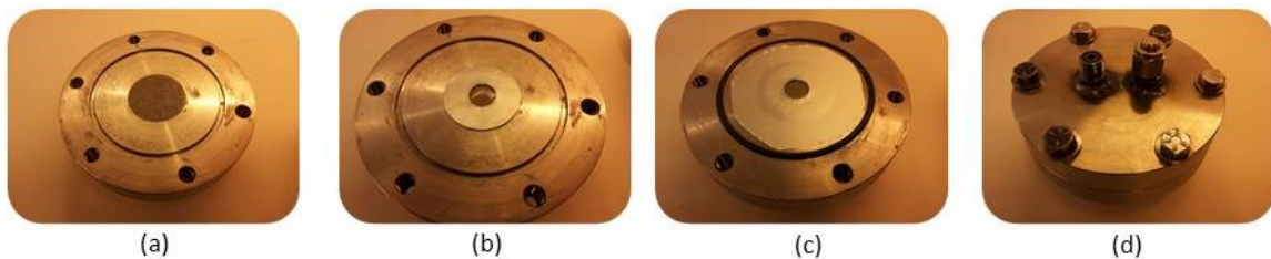
Figure 6.8 Mounting of membrane in the module: (a) the support for the membrane with a metal sinter in the middle, (b) the membrane is masked with aluminum tape on both sides and put on the metal sinter, (c) the masked membrane is glued to the test cell with aluminum tape, and (d) the top and the bottom of the module are put together
