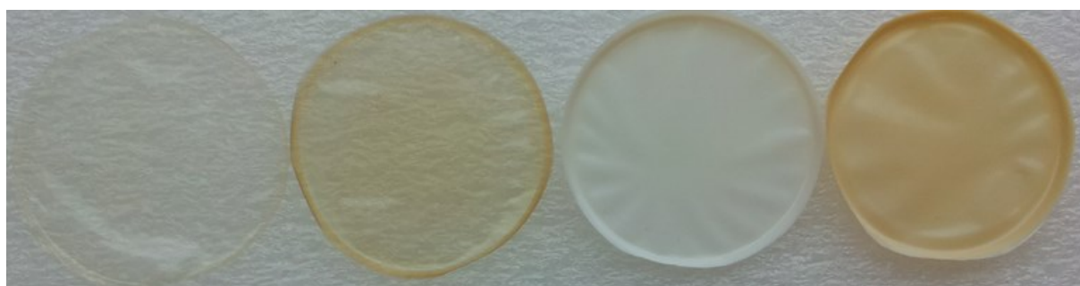
Figure 7.1 Photograph of membranes containing PTMSP. Membrane from left: pure PTMSP, 3wt% BAA, 20wt% TiO 2 nanoparticles, and 3wt% BAA + 20wt% TiO 2 nanoparticles in the last one to right.
