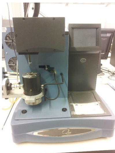
Figure 6.10 TGA Q-500 used in the laboratory
