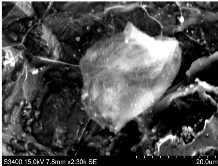
**Figure 8-26.** SEM showing typical goethite phase of corrosion product
