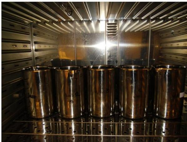
**Figure 7-5.** The inside of the Memmert<sup>®</sup>600 thermostat chamber at 135°C with the containers for the 5 different weeks of exposure shown.
