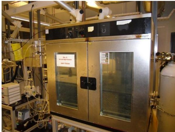
**Figure 7-2.** A Memmert® 600 thermostat chamber at 135°C ready to be used for the experiment
