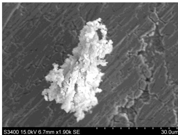
**Figure 8-27.** Flaky, porous and layers on metal surface as revealed by SEM
