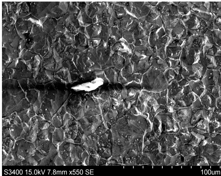
**Figure 8-25.** Lepidocrocite phase feature of corrosion products via SEM
