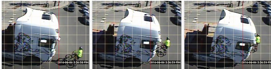
Figure 26 – Conflict between truck and cyclists (obvious from the truck cab's vertical movement caused by excessive braking manoeuvre), captured by camera's position #1
