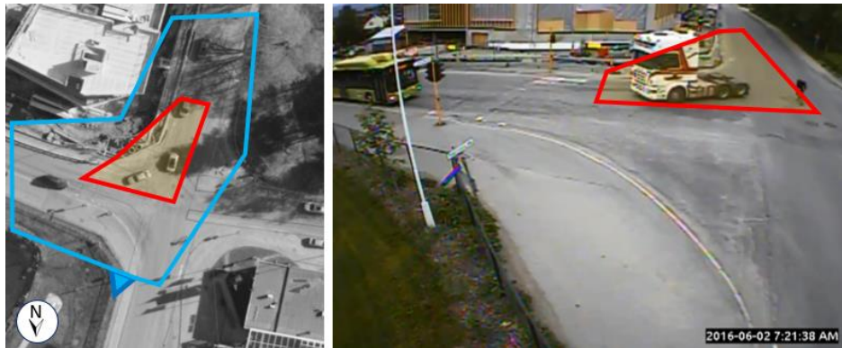
Figure 15 – Position of the camera (blue triangle), the camera coverage (blue) and the observed approach (red)
