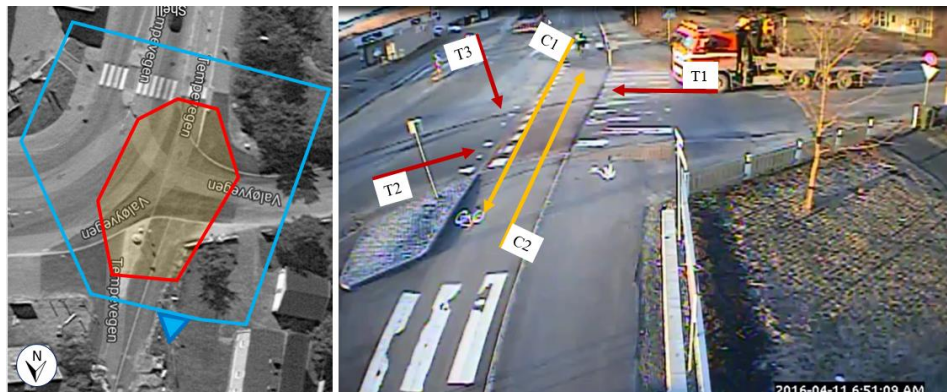
Figure 27 – Position of the camera (blue triangle), the coverage area (blue), observed approach (red) and observed directions (C=cyclist, T=truck)
