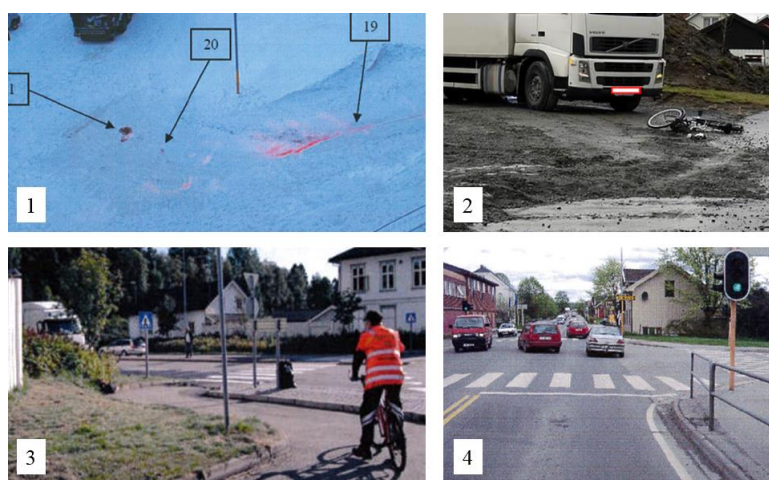
Figure 11 – Examples of the risk factors in fatal TCA in Norway - lack of winter maintenance (1), insufficient safety management in proximity to a construction site (2), visibility limited by greenery (3) and lack of dedicated cycle infrastructure (4) (source: NPRA reports)
