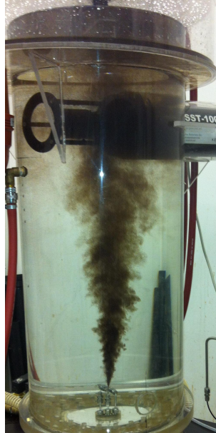
Figure 1.1: Illustration of an oil plume from SINTEF MiniTower (Brandvik, SINTEF, 2013).
