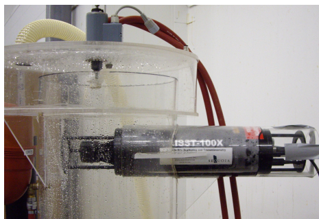
Figure 4.4: Placement of LISST-100X in the MiniTower (Lindersen, 2013).
