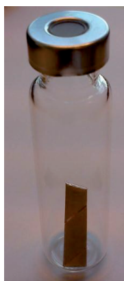
Figure 2. Glass vial with a piece of copper winding wrapped with paper (one layer).
