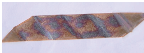
Figure 1. Insulating paper with Copper-Sulphide depositions.
