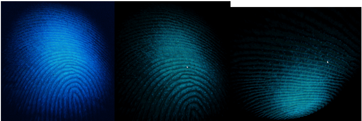
Fig. 4. thumb scan: 2x2cm area, 1408x1408x1024, 14.2 \mu m - surface fingerprint & sweat glands - transparent 3D visualization
