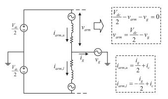
Fig. 2. Simplified MMC circuit, deriving  $v_{arm}$  and upper and lower arm currents
