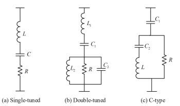
Fig. 5. Different resonant filter arrangements
