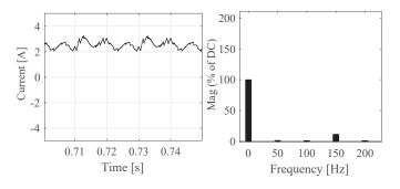
Fig. 11. Waveform and FFT of battery current with injected circulating current and passive interface filter
