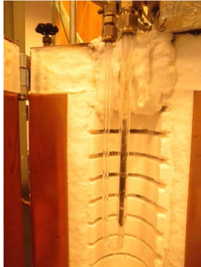
Figure 31: Catalytic reactor at the end of the activity test
