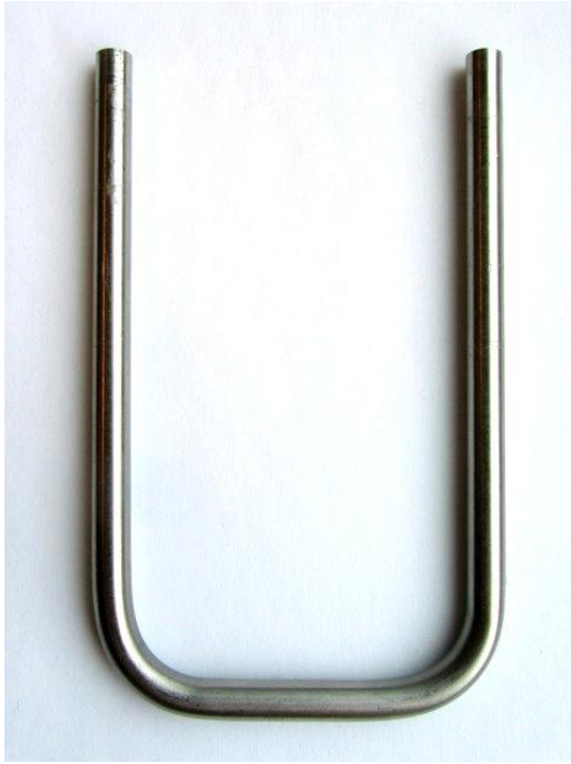
Figure 23: U-shaped tube. When heated internally by water, a heated surface is created
