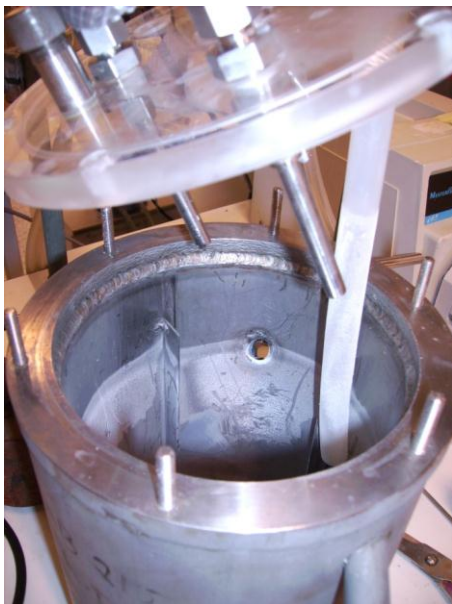
Figure 24: Scale depositions in reactor after completed experiment
