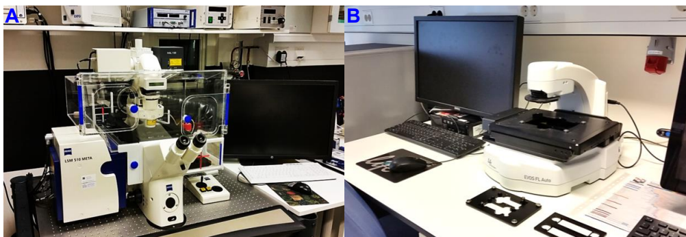
Figure 3.1.1.11 A) Zeiss LSM 510 inverted confocal microscope. B) EVOS FL Auto Cell Imaging System (Invitrogen).
