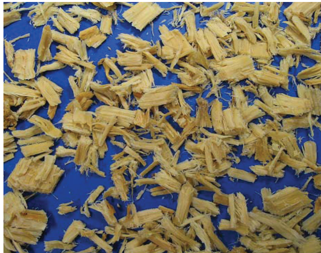
Figure 2.4: White spruce wood chips after pre-treatment in an Impressafiner (temperature 111°C, retention time 15 s, compression ratio 5:1).
