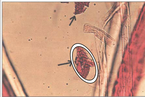
Fig 2. Pitch agglomerates in a machine chest stock sample (adapted from Laubach and Greer 1991).
