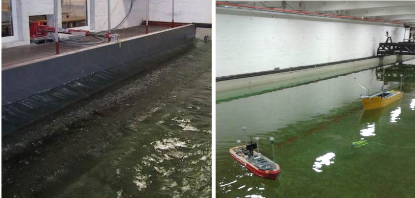
Figure B.4: (left) DHI wavemaker and (right) marine operation in the MCLab featuring Cybership 3 on DP, Cybership Enterprise in front to the left, and a remotely operated vehicle (ROV) Neptunus designed and built by students under water between the surface models.
