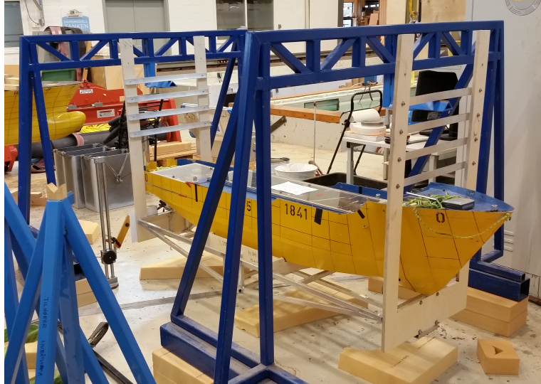
Figure B.2: Cybership 3 during oscillation tests in roll.
