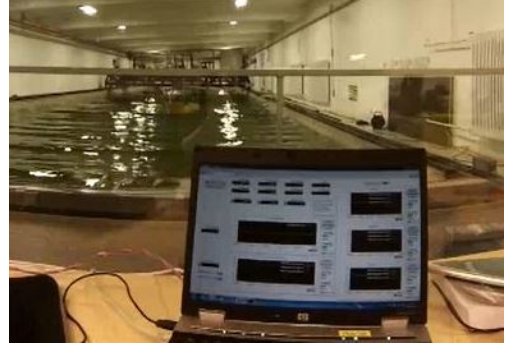
Fig. 4. Operator laptop where DP setpoints and controller gains are specified. The wave flap is also seen directly behind the laptop.
