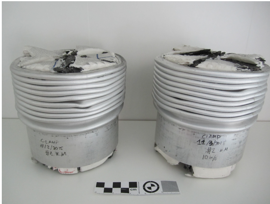
Figure 15: Components D1 (left) and D2 (right) after impact test at 10 m/s. The clamped length of 50 mm is clearly appreciable.
