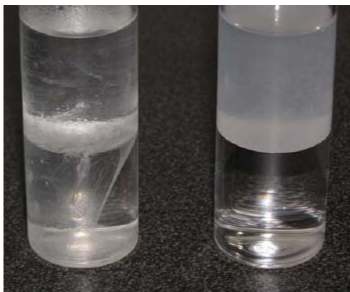
Figure 2.6 Calcium naphthenate of C 80 naphthenic acids (left) and of p-(n-dodecyl) benzoic acid (right).
