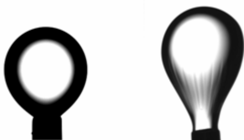
Figure 5.10 Contracted oil drops covered with C_{80} naphthenic acids (left) and calcium naphthenate (right)
