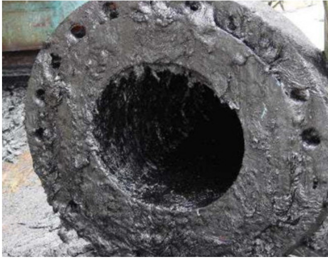
Figure 1.10: Asphaltene deposition in a pipeline [20].
