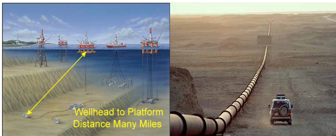
Figure 1.5: Figure to the left shows typical tiebacks from wellhead to the platform. For successful transport of produced fluids knowledge about “flow assurance” is important [13]. Figure to the right shows oil pipeline in Saudi Arabia [14].
