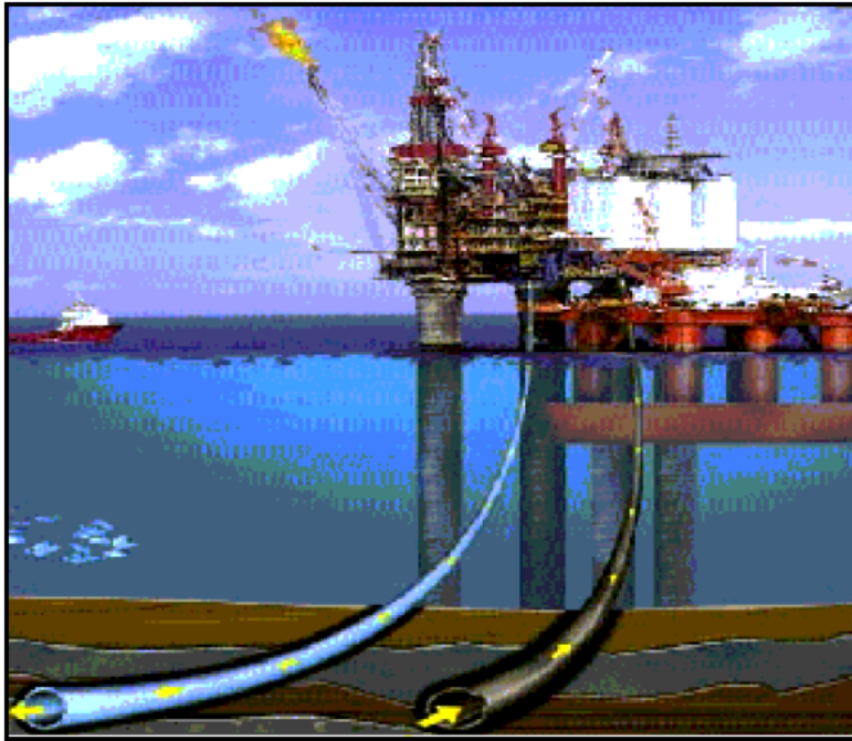
Figure 3.1: Re-injection of separated water from an offshore installation [3].
