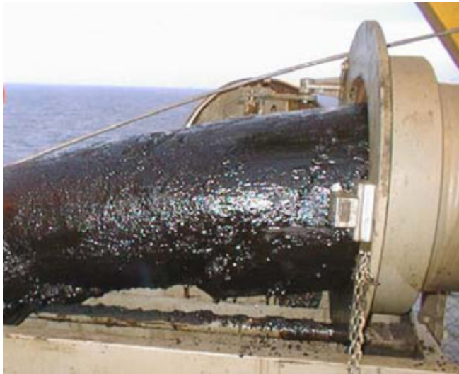
Figure 1.9: Pigging to remove wax from a subsea transfer line. Pigging devices fit the diameter of the pipe and scrape the pipe wall as they are pumped through the pipe [20].
