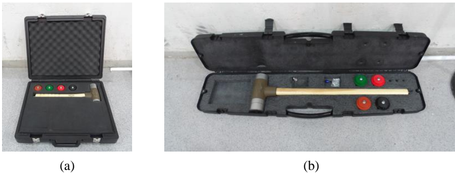
Fig. 5.3 Modal hammer; a) Heavy Duty Type 8208; b) Heavy Duty Type 8210.
