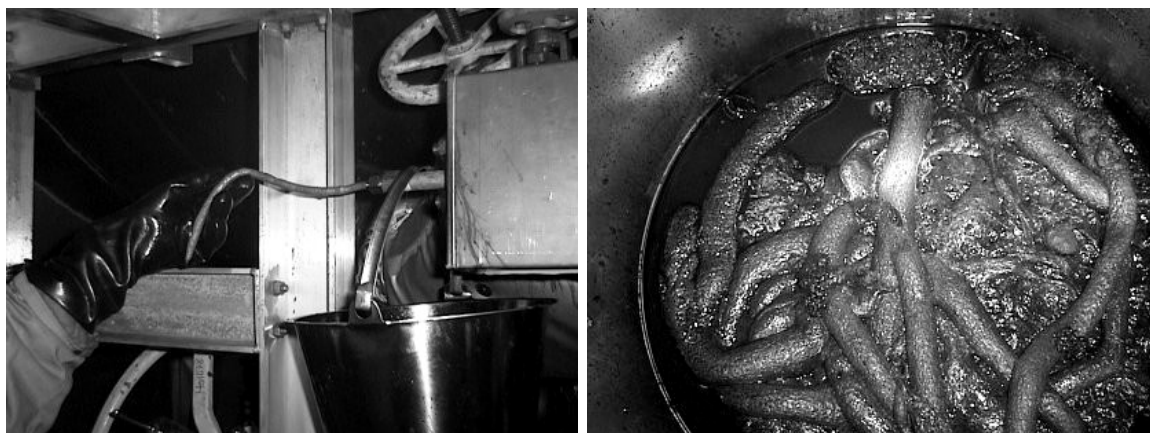
Figure 5.1 Calcium naphthenate deposit (right picture) collected from an o/w-separator. The outlet of the separator (left picture) is located at the o/w-interface. [Pictures, by courtesy of Statoil ASA]
