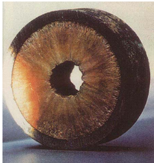
Figure 3-2 Cross-sectional view of a plugged pipeline [3]
