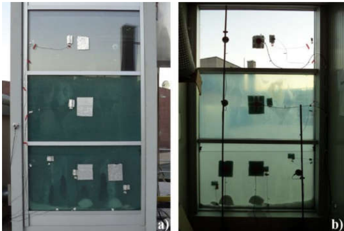
283 284 Figure 2 – Test cell with sensors: a) external view; and b) internal view.
