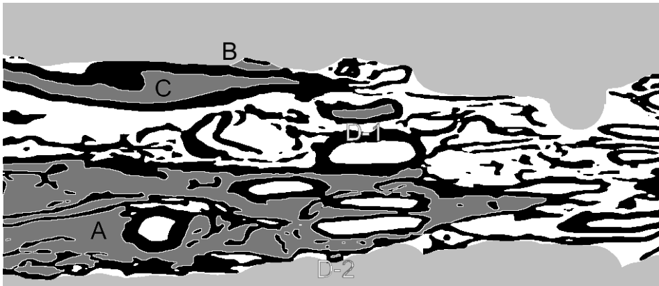
Figure 4.17 Illustration of pore areas with different characteristics in a typical cross section in the newsprint sample. Pore area A is large and branching limited by solid elements, image edge and defined sheet surface. Surface pore area B is limited by solid elements and the defined surface. Image edge pore area C is limited by solid elements and the image edge. Enclosed pore areas D-1 and D-2 is limited only by solid elements.
