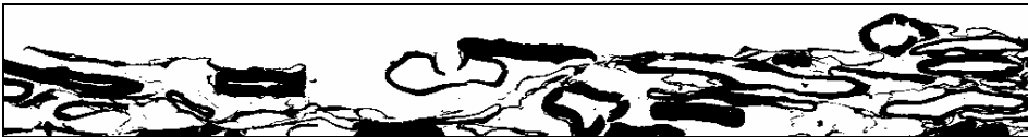
Figure 2.6 The surface of a typical cross sectional image of a newsprint sample. On micrometer scale the surface is rough and discontinuous.
