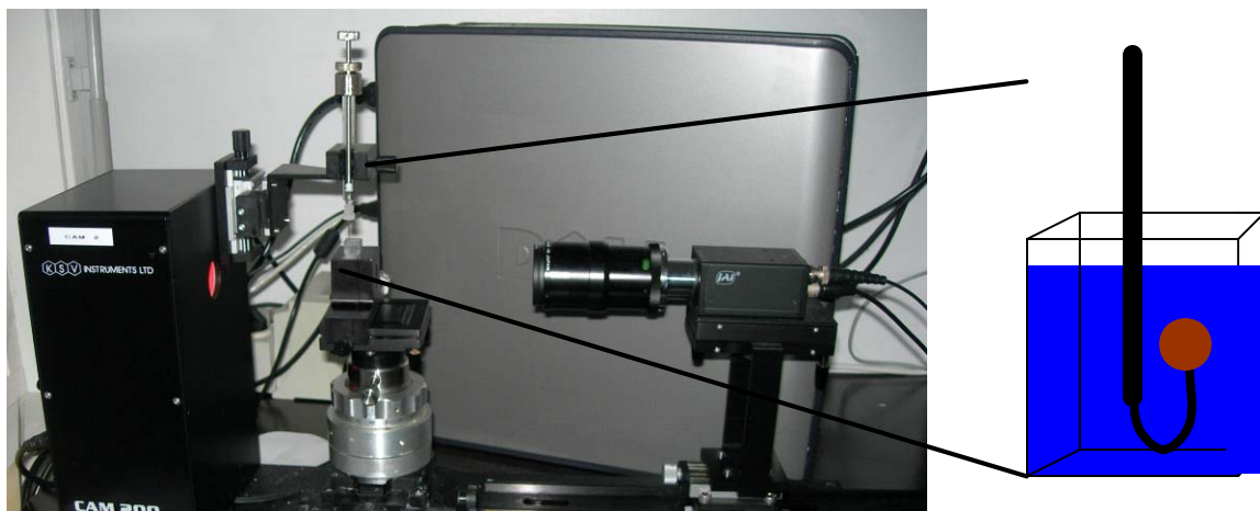
Figure 5-13. Setup of the CAM 200 from KSV Instruments. A syringe with the oil phase is placed in a quartz crystal container containing the water phase. A (high speed) camera takes pictures of the droplet. The interfacial tension is calculated from the shape of the droplet and the difference in density between the two phases.
