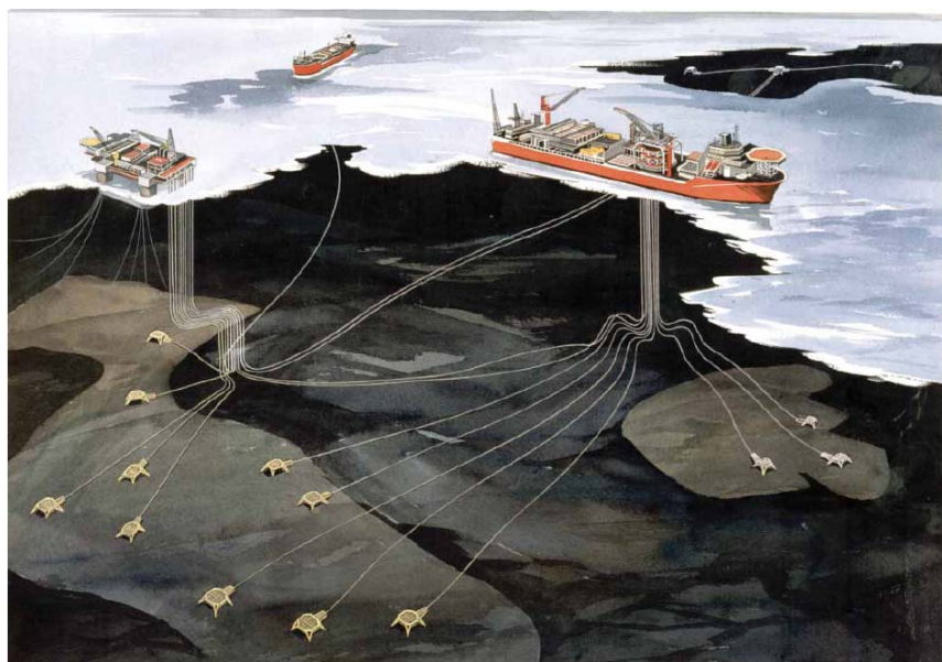
Figure 1-6. The Statoil operated Åsgard 'field', showing sub sea well templates linked by multiphase flow lines and risers to the Åsgard B floating production platform (left) and the Åsgard A floating production, storage and offloading ship. 7
