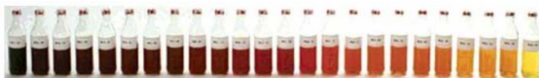
Figure 2-1. Crude oils are seen as black fluids for the most part, but this picture shows the separation of the crude oil due to gravity in the well. The dark oils (left) are higher in density and has higher concentrations of asphaltenes and other poly aromatic hydrocarbons (PAH). 11
