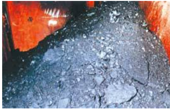
Figure 2-7 Asphaltene debris dug out from a separator. 7
