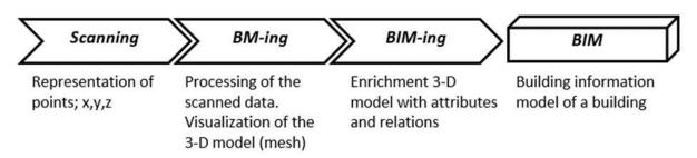
Figure 4: Main stages in the scan-to-BIM process. (Source: Hjelseth et al, 2016)
