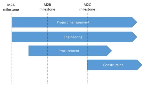
Figure 3: Parallelism between engineering, procurement and construction. (as published by Mejlænder-Larsen (2016))
