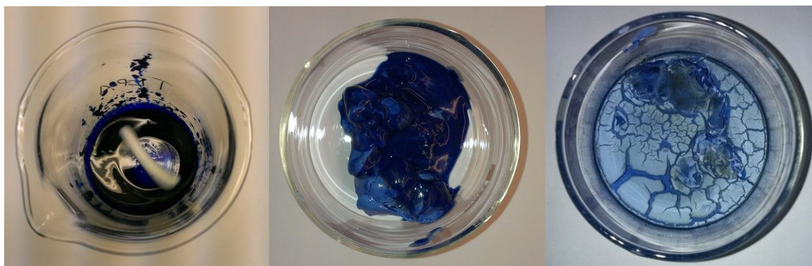
Figure 3.2: Different steps of the synthesis; on the left is the Cu-TEPA mixture while stirring, the middle shows the gel after hydrothermal treatment and the right is after washing and drying.
