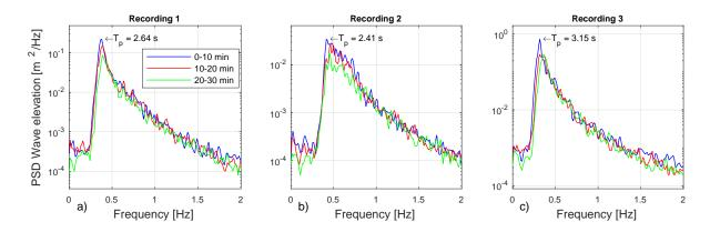
Figure 8: PSD of the wave elevation for the three recordings taken from the midmost wave radar.
