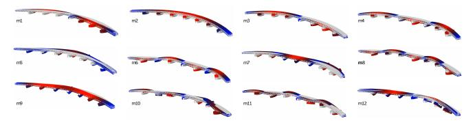
Figure 5: Twelve of the mode shapes from the system model used for the input and state estimation.
