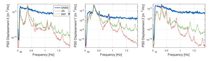
Figure 19: PSDs of the estimated displacements in recording 1 compared to GNSS measurements.
