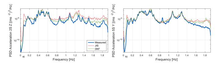
Figure 15: PSDs of the estimated acceleration response in recording 2 compared to the measured reference.
