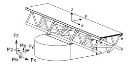
Figure 6: Sketch of the modelling of the wave forces on the pontoons.
