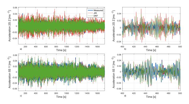
Figure 14: Estimated acceleration response in recording 2 compared to reference measurements.
