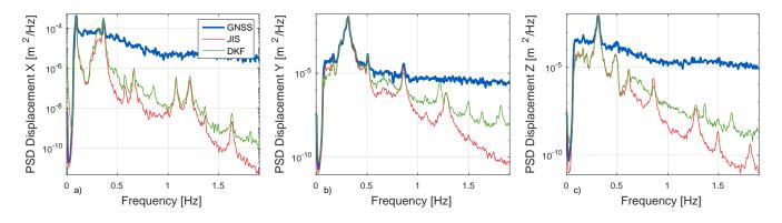
Figure 21: PSDs of the estimated displacements in recording 3 compared to GNSS measurements.
