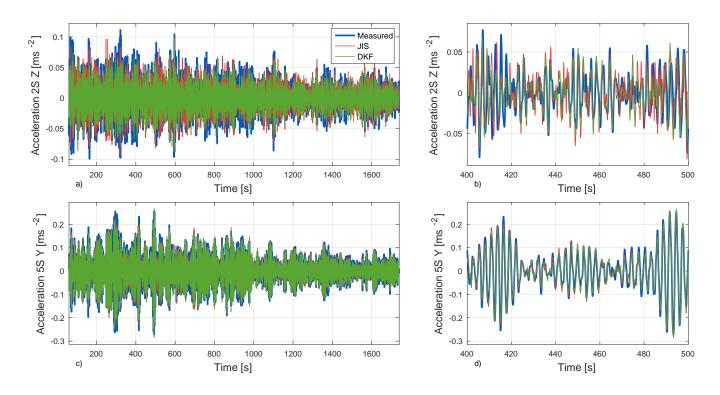
Figure 12: Estimated acceleration response in recording 1 compared to reference measurements.
