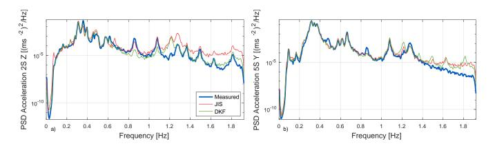
Figure 17: PSDs of the estimated acceleration response in recording 3 compared to the measured reference.
