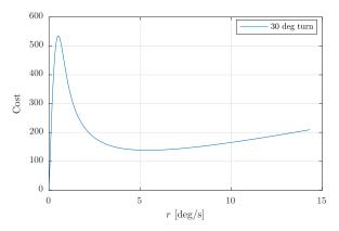
Fig. 5: Cost of performing a 30 deg course alteration, using different ROTs. The peak at  $r \approx 0.51$  deg/s is the highest cost, while r = 5.42 deg/s is the minimum after the peak.
