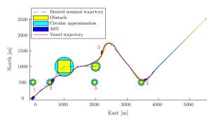
Fig. 6: Simulation result using the quadratic objective function  $\phi_1$ . Note that the size of the ownship (in blue) is overexaggerated for visibility. Hence, what appears to be a collision with the moving obstacle is in fact not a collision.
