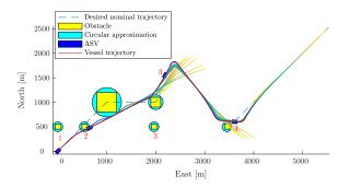
Fig. 7: Simulation result using the modified objective function  $\phi_2$ . Note that the size of the ownship (in blue) is overexaggerated for visibility. Hence, what appears to be a collision with the moving obstacle is in fact not a collision.
