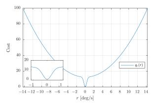
Fig. 4: ROT penalty function with  $a_r = 112$ ,  $b_r = 6.25 \cdot 10^{-5}$  and  $r_{\rm max} = 0.25$  rad/s  $\approx 14.3$  deg/s. The function is nonconvex close to the origin, but remains smooth as the zoomed insert shows.
