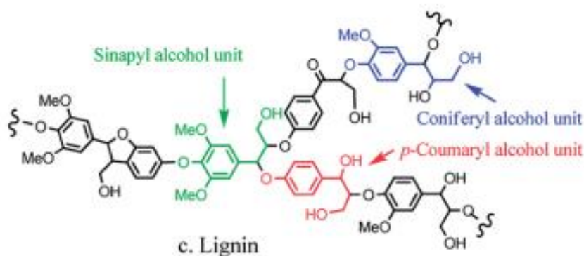
Figure 3: Schematic structure of lignin indicating the three main units (Adapted from [2]).
