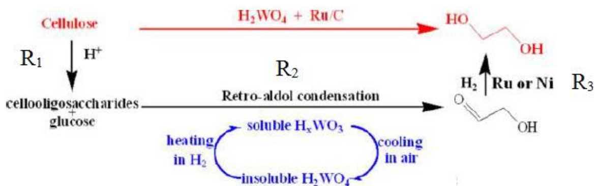
Figure 11: Reaction pathway scheme for cellulose conversion to EG over tungsten based catalysts (Adapted from [7]). The red part represents the overall reaction, the black part represents the three consecutive reactions towards EG, and the blue part represents the temperature controlled phase transfer behaviour of tungsten acid.
