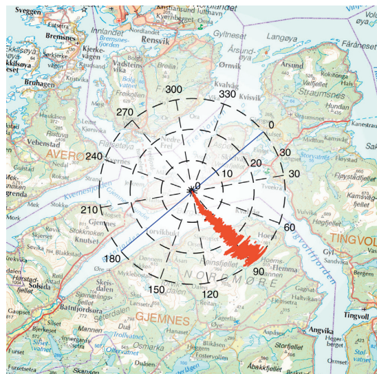
Fig. 4. Wind direction time evolution for wave-driven recording. The blue line indicates the tangent at the midspan of the bridge. The plotted wind direction corresponds to the average of anemometers A2 and A3, and indicates the origin of the wind. The amplitude axis corresponds to the time in minutes. (For interpretation of the references to colour in this figure legend, the reader is referred to the web version of this article.)
