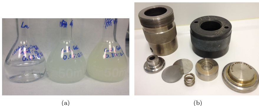
Figure 3.1: 3.1(a): Flasks of 0.03M, 0.15M and 0.30M precursor concentrations. 3.1(b): 4746 High Strength Acid Digestion Vessel (autoclave) with all parts, including corrosion and rupture discs.
