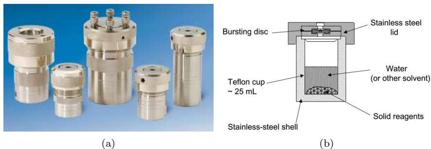
Figure 2.24: 2.24(a): Autoclaves of varying designs, volumes and pressure limitations. The picture is taken from the Parr Instrument Company website. 76 2.24(b): The cross section of an autoclave with liner, filled with reagents and water. 75
