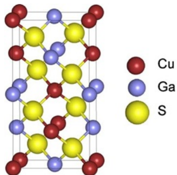
Figure 2.13: The tetragonal unit cell of \text{CuGaS}_2 . 50
